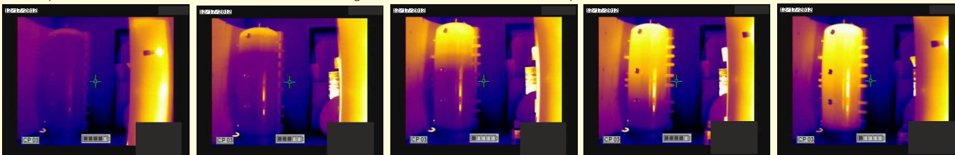
These pictures show the stratification inside of the Logix24 when connected to a solar plant:
