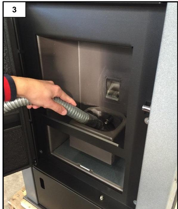
Thoroughly clean the brazier from combustion residues by taking it out from its position and removing any residues inside (Figure 2).
