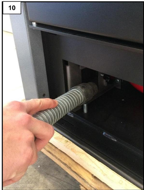
After unscrewing the hand-wheels, extract the side flue gas pass inspection vent (Figure 9). Remove the deposits inside using a suitable ash vacuum device (Figure 10). When finished, close the pipes making sure that you have secured the two inspection openings. Replace the front panel below.
