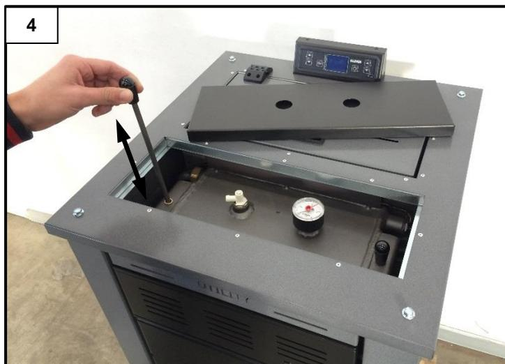
Press repeatedly (from bottom to top and vice versa for the entire length of the rod) the two side scrapers to allow cleaning of the side flue gas pass (Figure 4).
