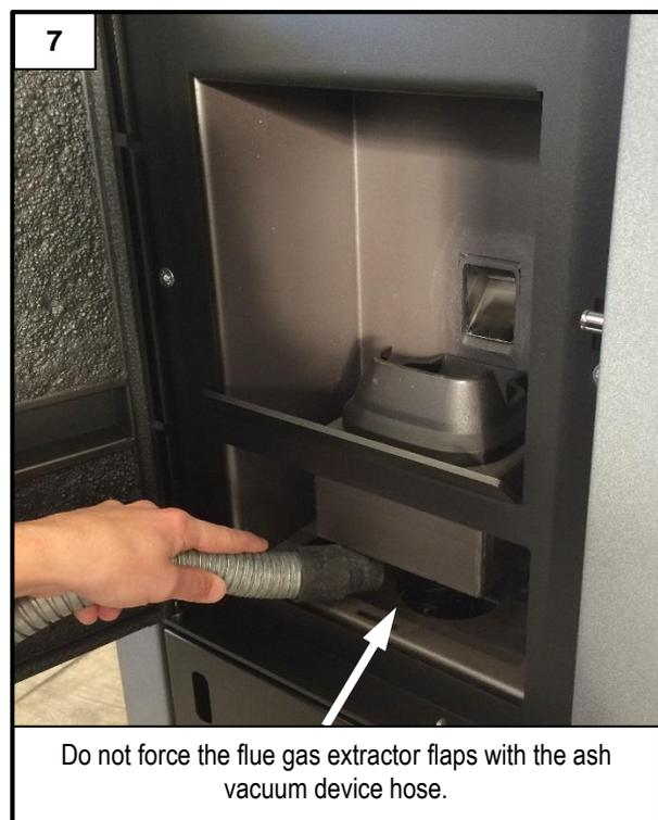
After removing the ash drawer pull out the bottom under it (Figure 6) and vacuum the deposits on the inside using a suitable ash vacuum device (Figure 7). When finished, replace the bottom and the ash drawer.
