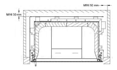
ATTENTION, THESE DIMENSIONS DO NOT INCLUDE THE REQUIRED THERMAL INSULATION. THEY ARE TO BE MARKED UP BY THE THICKNESS OF THE INSULANT.
