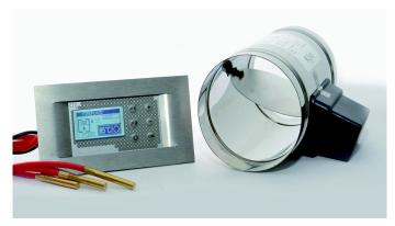
Connecting an AirSmart controller and vent is a way to avoid potential ventilation problems. A door sensor is fitted to the stove and whenever the door is opened the controller opens a sealed vent to the room to supply extra fresh air. If there is a powercut then the vent is also opened as an additional
