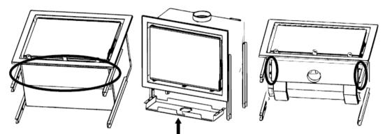
**Direct air kit for Octave 70i and 90i.** This optional kit enables you to bring the combustion air from the outside and will require the stove to be installed with a space underneath. This is best achieved using the adjustable legs kit (see below).
