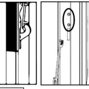
**Door closing adjustment.** On all the Octave models you can adjust the door using the bolts in the front. Tightening or loosening these bolts will ensure the correct adjustment.
