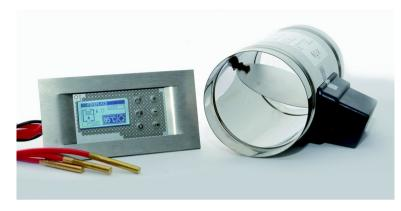
Connecting an AirSmart controller and vent is a way to avoid potential ventilation problems. A door sensor is fitted to the stove door and whenever the door is opened the controller opens a sealed vent to the room to supply extra fresh air. If there is a power cut then the vent is also opened as an additional safety feature. The AirSmart controller can be a stand-alone unit, or combined with a full automated stove
