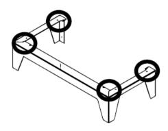
**Octave 70F Stand positioning**. Support the stove over the stand, lining up the six holes in the stove and stand. Bolt the stove and stand together using the six bolts supplied.
