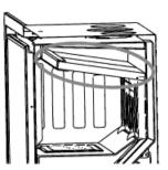
On the Octave 90i DS the baffle plate set consists of the deflector bricks and tertiary combustion tube. The RHS bricks should be positioned first, then insert the RHS end of the baffle set as far as it will go above the
