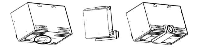
iii) Using the bolts supplied, connect the box to both the base and the rear of the stove.
