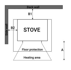
Here are the minimum distances which must be kept between the stove and combustible walls and other combustible materials.
