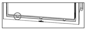
The **tertiary air** control lever is situated under the door on the left hand side. The amount of air entering the stove increases when the lever is moved in the direction of the large side of the triangular cut-out on the lever.
