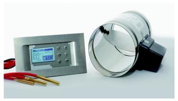
Connecting an AirSmart controller and vent is a way to avoid potential ventilation problems. A door sensor is fitted to the stove and whenever the door is opened the controller opens a sealed vent to the room to supply extra fresh air. If there is a powercut then the vent is also
