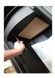
Using a 5mm hex key, unscrew the second baffle and it's bracket being careful to support its weight whilst removing.
