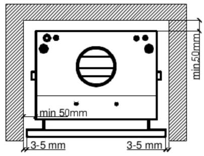
Ensure there is a minimum gap of 2 - 3mm between the firebox and the side wall at the frontal area of the boiler stove.
