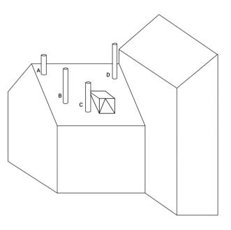
Termination/Cowl: The cowl terminates the chimney and it is recommended that an effective anti-downdraft cowl should always be used. It must have a usable outlet cross-section no less than double that of the flue onto which it is inserted. In must prevent rainwater or snow entry. It must be ensure the discharge of combustion by-products even in the event of winds from every direction and inclination.
