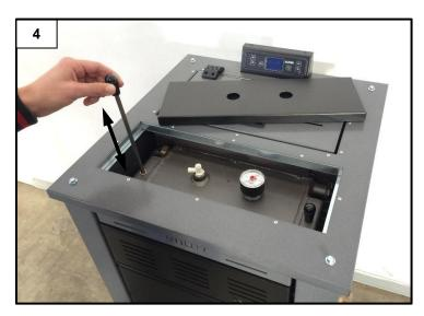
Press repeatedly (from bottom to top and vice versa for the entire length of the rod) the two side scrapers to allow cleaning of the side flue gas pass (Figure 4).
