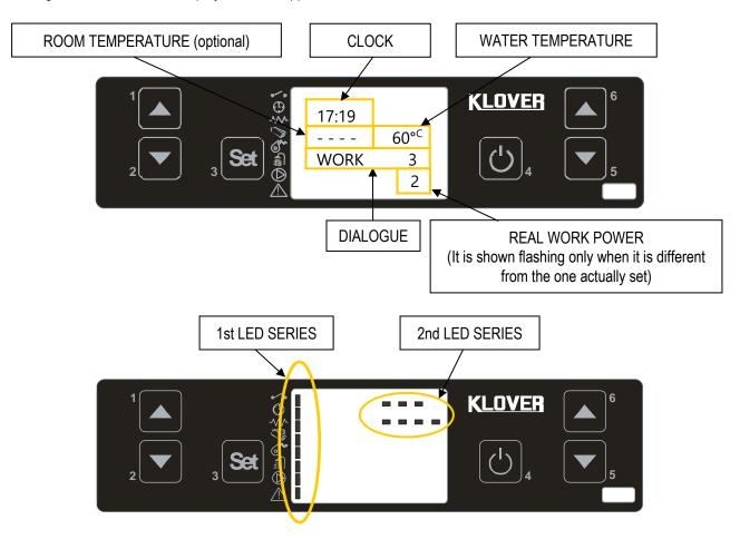
The following figure describes the meanings of the status signals appearing on the display left side (1st LED SERIES).
