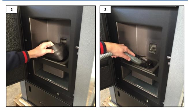
Thoroughly clean the brazier from combustion residues by taking it out from its position and removing any residues inside (Figure 2).
