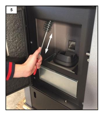
Clean the pipes inside the combustion chamber using the supplied brush and passing it repeatedly between one and the other pipe (Figure 5).
