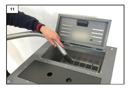
To ensure correct operation, it is necessary to remove the sawdust deposited on the base of the tank (Figure 11) at least once every 15 days. The pellet tank must be emptied at the end of every season.
