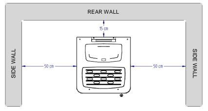
Any shelves or false ceilings mounted above the appliance must be at least 100 cm away from the top part of it. Furniture and movable objects must be positioned at least 15 cm from the side surfaces of the appliance; these objects must be moved when performing maintenance on the appliance.
