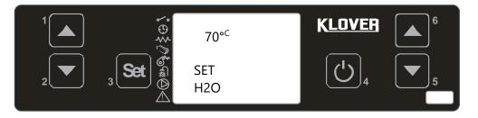
After setting the desired value, press button 4 or wait a few seconds to confirm.
