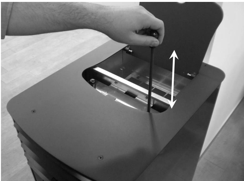
After opening the pellet loading door, pull the two underlying knobs to clean the rear flue gas circuit pipes.
