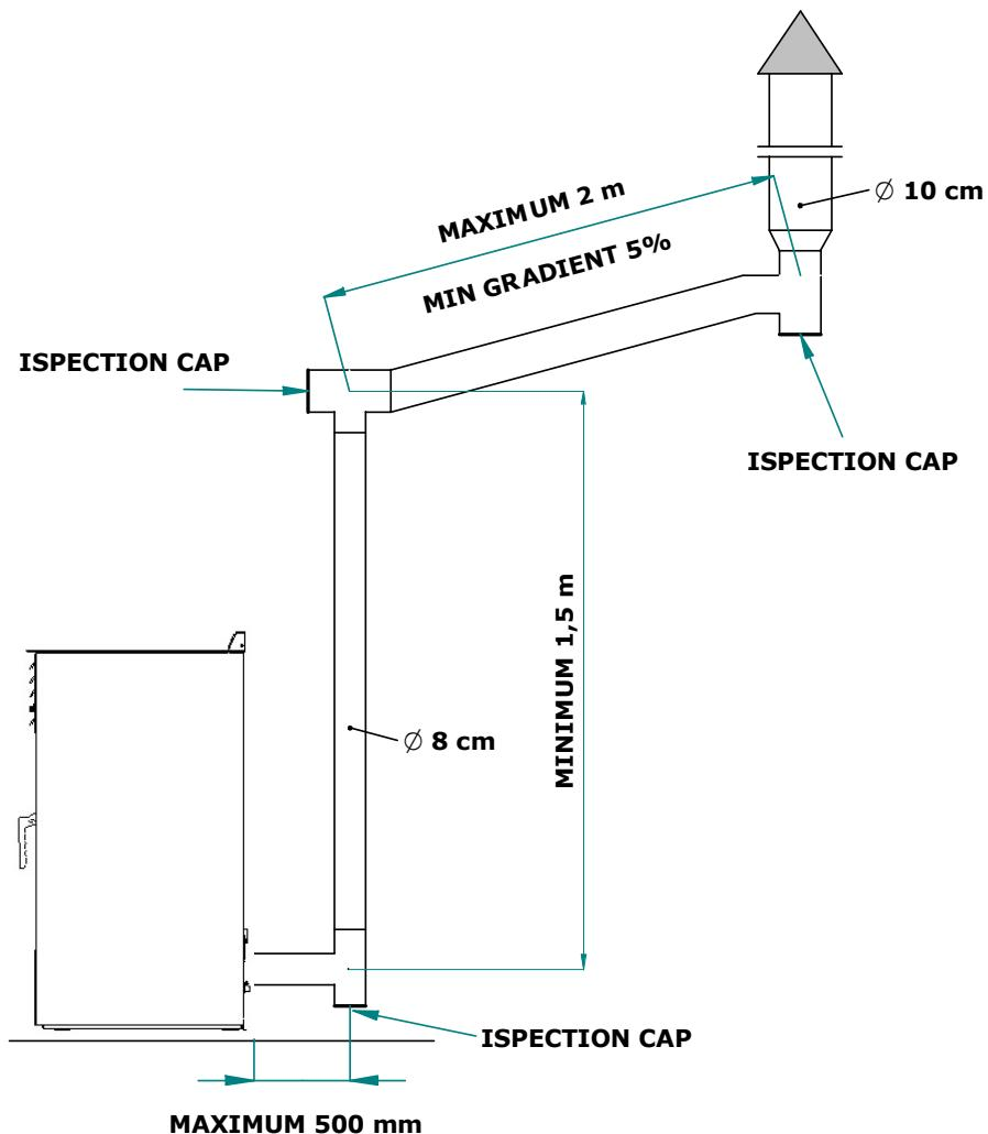
If a "traditional" flue is used for discharging flue gas, make sure that it is in good working order and that it complies with the applicable standards. **If the flue is too large (internal diameter greater than 14 cm), duct the flue using an appropriately insulated stainless steel pipe (using rock wool or vermiculite) sized according to the relevant route. The connection to the flue must be appropriately sealed.**
