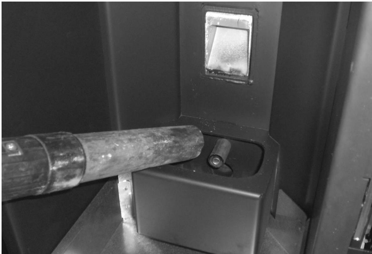
Use an ash vacuum cleaner to remove any ash deposited under the brazier.
