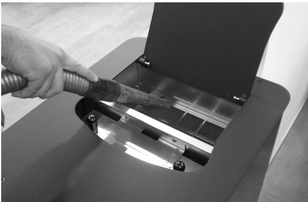
To ensure correct operation, it is necessary to remove the sawdust deposited on the base of the tank at least every 15 days.
