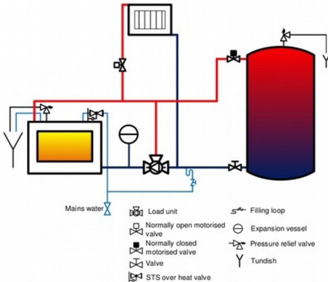
*Illustration 2* is a suggested typical plumbing schematic showing the boiler stove connected to a thermal store. The positioning of the pipes for the heat leak radiator around the load unit is very important. In the LK 810 ThermoMat range, the gravity circuit
