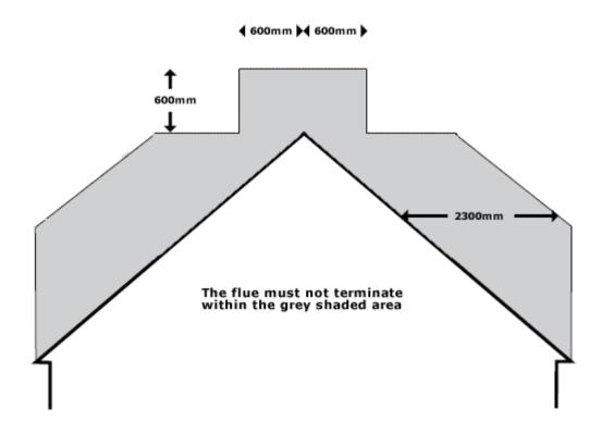
The grey area in the picture shows where the flue must not terminate on a roof with standard (non flammable) roof material.
