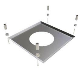
2 PC ROUND FIXED FINISHING PLATE 90 DEGREE Code:15-\*\*\*-118 150mm wide. Covers any gap to combustibles, or making good around flue as it passes through ceilings or walls.
