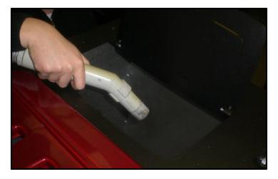
For correct functioning, it is necessary to use a suction device to remove the sawdust deposit on the base of the pellet tank at least every 15 days. The pellet tank must be emptied at the end of every season.
