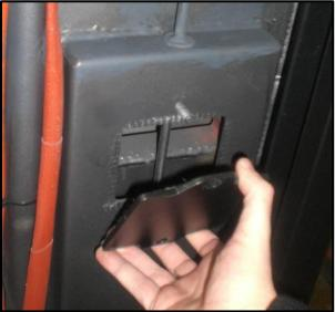
After having loosened the two bolts, remove the lateral flue gas pass inspection outlet (pellet side).
