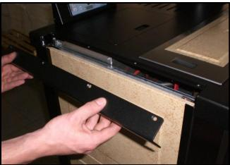
Loosen the four screws in the upper left angle.
