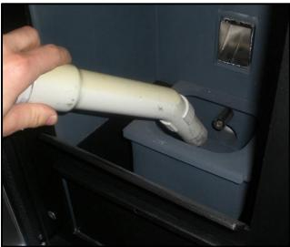
Clean the brazier from combustion residues, by removing it from its seat. Use a suction device to remove the ash that is deposited under the brazier.
