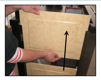
After having removed the upper left angle, slide the three lateral majolicas upwards (or the painted steel side).
