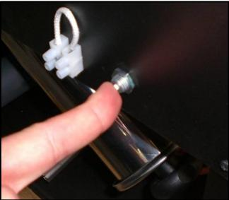
Loosen the black cap behind the thermo stove and press the button under the cap. At this point, the thermo stove can be switched back on.
