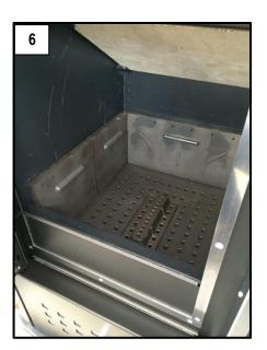
Remove the refractory brick above the combustion chamber (figure 4) and clean the upper flue by passing the supplied brush repeatedly between the pipes (figure 5). Once clean, reverse the above procedure, carefully replacing all the parts previously removed, paying particular attention to repositioning the cast iron grate as shown in the photo above (figure 6) to prevent ash from compacting and falling into the ash drawer, which would reduce the flow of combustion air.
