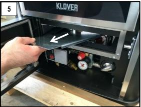
After removing the ash drawer (figure 4) pull out the bottom (two pieces) (figure 5).
