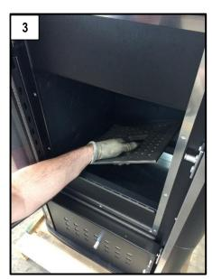
Remove the five cast iron partitions inside the combustion chamber (figure 1). Next, remove the cast iron grate (figures 2 and 3). Remove any deposits from the walls of the combustion chamber.
