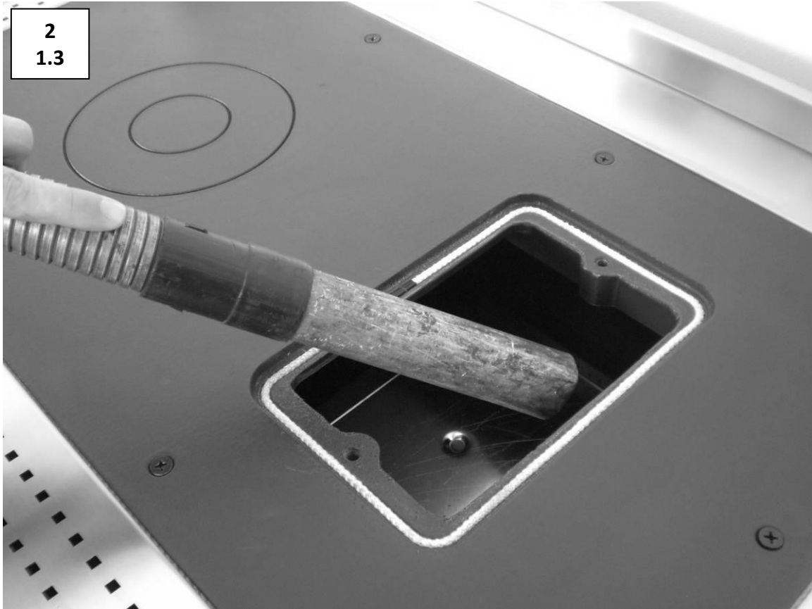
Dismantle the outlet on the cooking plate and suck the ash deposit above the oven. Properly re-position the outlet after cleaning ensuring it is flue gas sealed.
