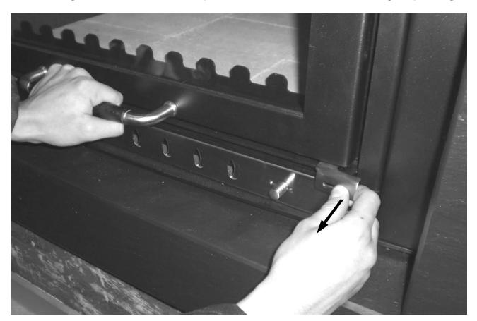
To open the hinged door you should release the designated hook as shown in the photo. The vertical sliding door must be open.
